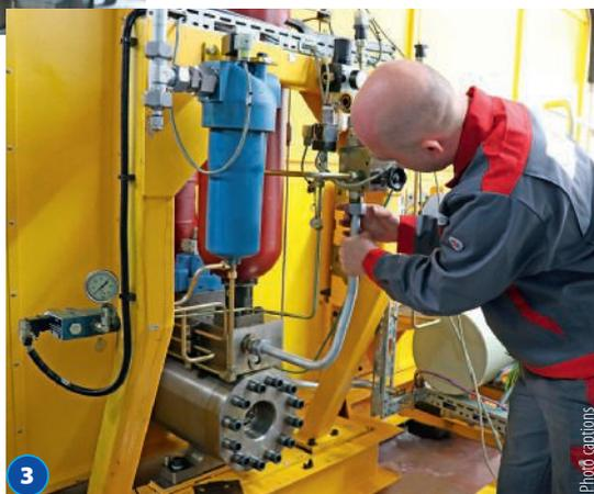
3 The tasks of ASK at the Stauff Development Centre also included assembly of the tubes
