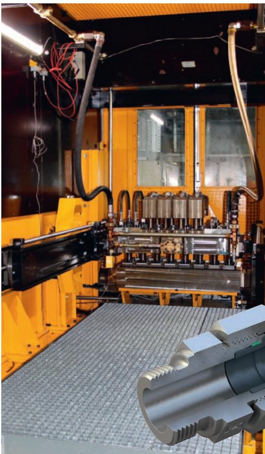
With the pulse testing system, Stauff carries out “Omega tests” on hoses to test their service life under bending and pressure change stress
